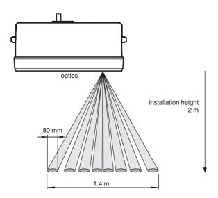
The ProScan is a 12-beam energetic light scanner based on the principles of active infrared. The beams, which are switched independently, enable the sensor to fan out across an extremely wide and narrow detection field in the area of the door.
